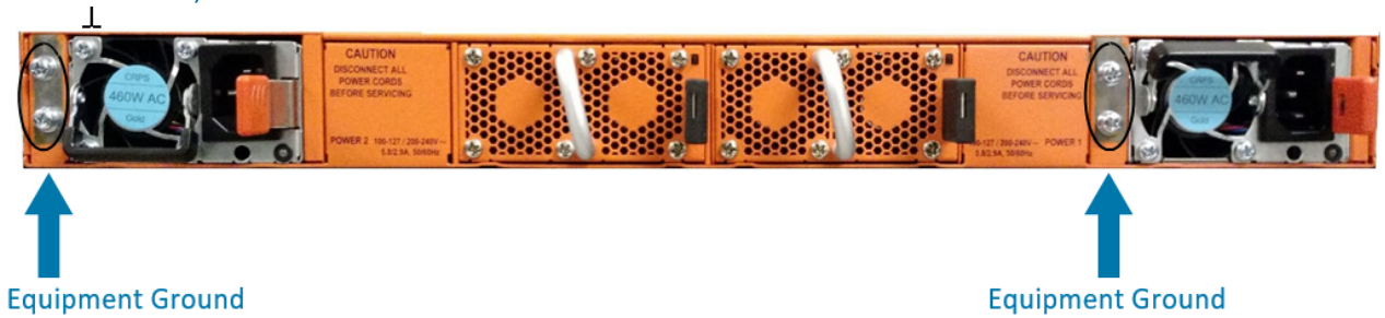
Figure 14 Ground Screws (GigaVUE TA Series-TA10 Shown)
